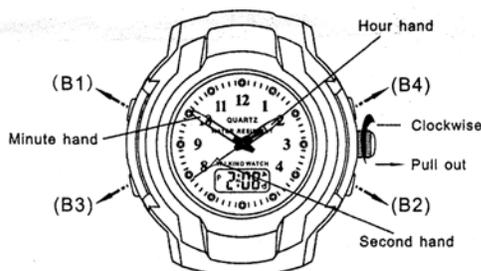
Gently pull out the crown, then adjust the exact analog time by turning the crown clockwise. Push the crown in after finishing the adjustment (see diagram above).
